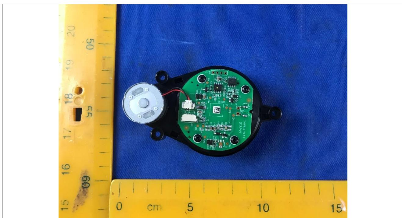
Details of: Internal view for radar module
