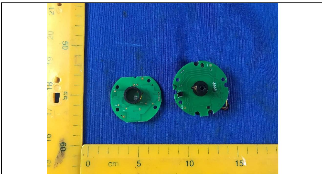
Details of: PCB view for radar module
