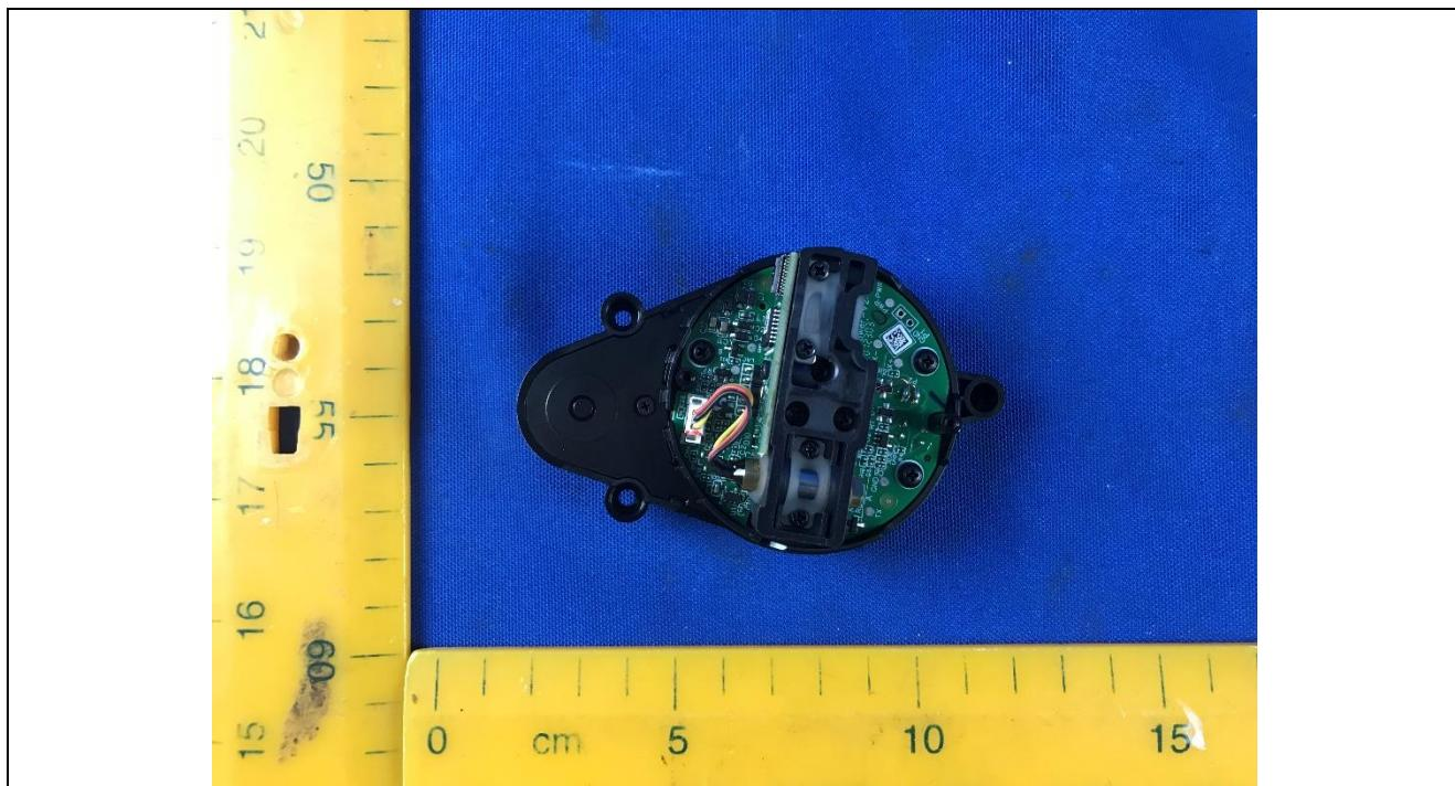
Details of: PCB view for radar module
