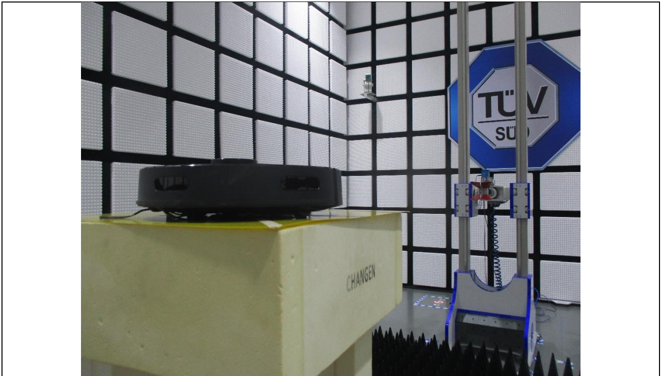
Radiated Emission test (1000MHz to 18000MHz)
