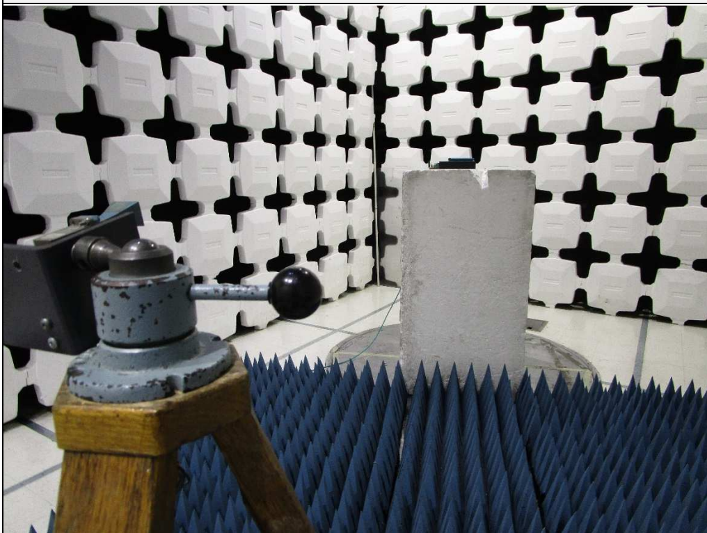
Test Setup for Spurious Radiated Emissions, 26.5GHz – 40GHz – Antenna Polarization Vertical
