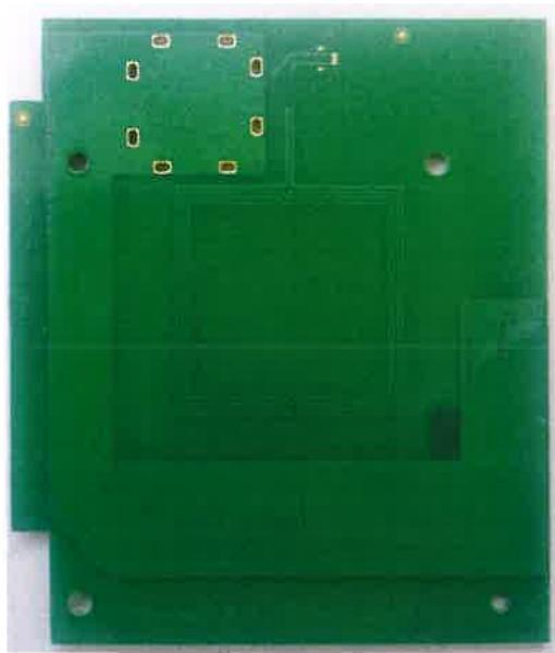
The antenna is made of a spiral loop (single loop antenna) and permanently connected to the 13.56MHz NFC controller through a PCB trace.
