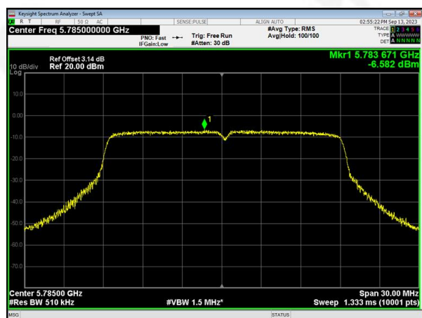
(802.11ac20) PSD plot on channel 157
