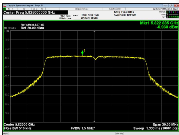
(802.11ac20) PSD plot on channel 165
