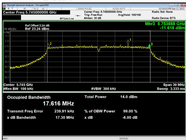
(802.11n20) 6dB Bandwidth plot on channel 165
