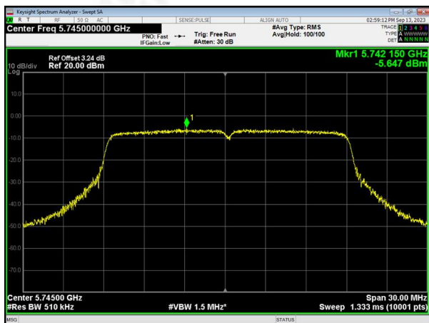
(802.11n20) PSD plot on channel 149
