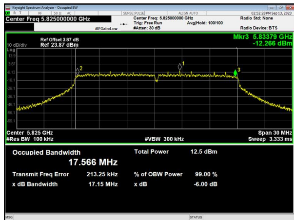
(802.11ac20) 6dB Bandwidth plot on channel 165
