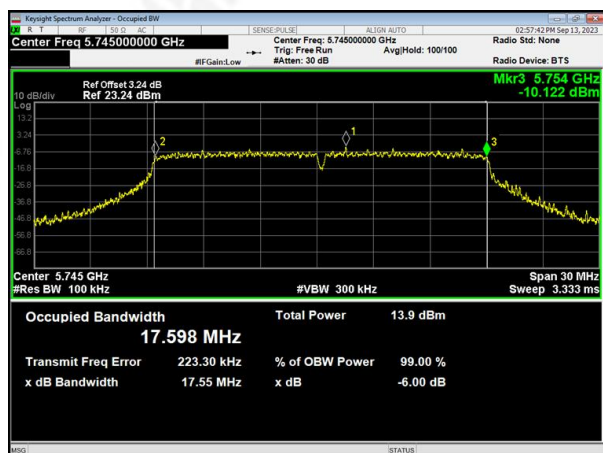
(802.11ac20) 6dB Bandwidth plot on channel 149
