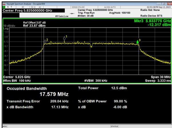
(802.11n20) 6dB Bandwidth plot on channel 165
