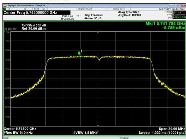
(802.11ac20) PSD plot on channel 165
