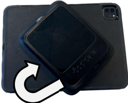
A magnet will help guide the two pieces into place. Once in place, rotate the Kora to the right.
