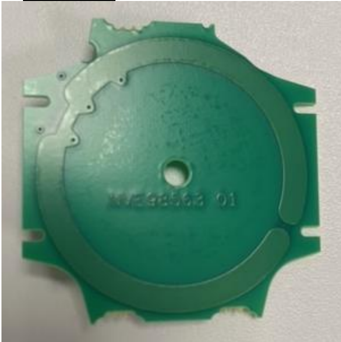
Coil side of the antenna board
