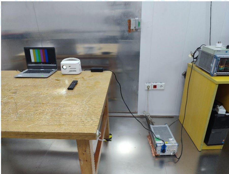
Photo of Setup for Conducted Emission
