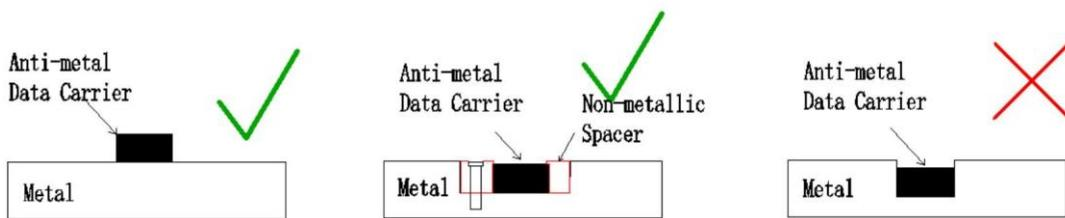
Note: If it is directly embedded in the metal installation, please make sure that the surface of the data carrier is not lower than the metal surface, otherwise the reading distance will be greatly reduced.
