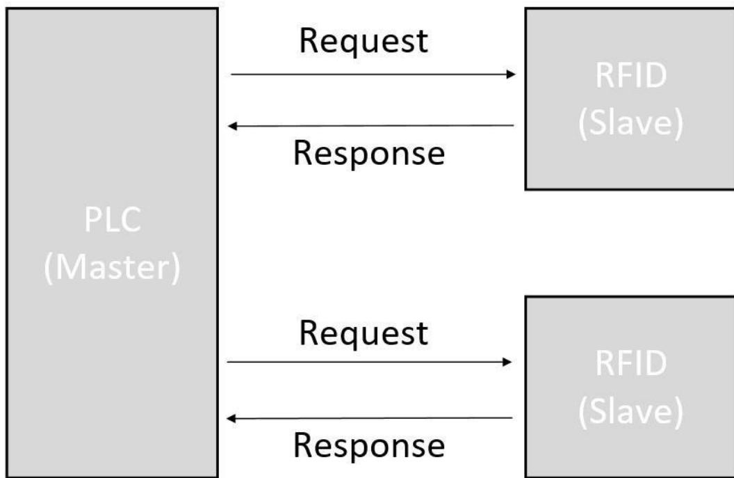
To establish communication, you need to pay attention to the device address and serial port configuration parameters. The default device address is 1, and the device address can be configured according to the actual situation during use. When there are multiple devices in the network, each slave device needs to be configured with a different address, and the master device controls each slave device through the address in turn. Multiple devices are connected to the serial network in parallel.
