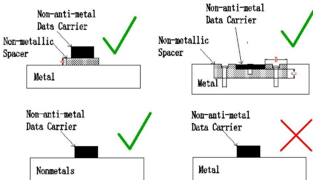
Non-anti-metal data carriers are installed in a metal environment, the following restrictions need to be met:
