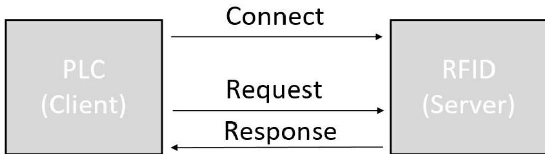
you need to configure the IP address. The default IP address of RFID is 192.168.0.10, and the fixed port number of MODBUS TCP is 502. Before establishing a connection, it is necessary to confirm that the PLC and RFID are in the same network segment. When multiple devices are connected to the network, each RFID needs to be configured with a different IP address, and multiple devices can be connected together through a switch.
