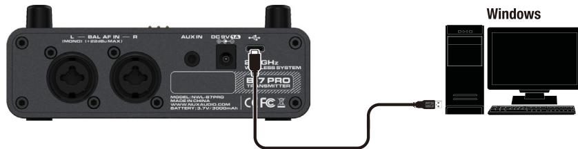
After you install the NUX ASIO Driver to your computer, you can connect the TX of B-7 PRO to your computer with a USB cable, you will find it as a USB audio device as below. Then you can start to record.
