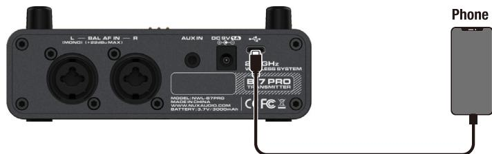
When connecting your smartphone to B-7 PRO for the first time, it may show two options on the phone's screen for you to choose. Please select the "USB headphones device". Or, you can check and setup "Connected To Headphones" as below.
