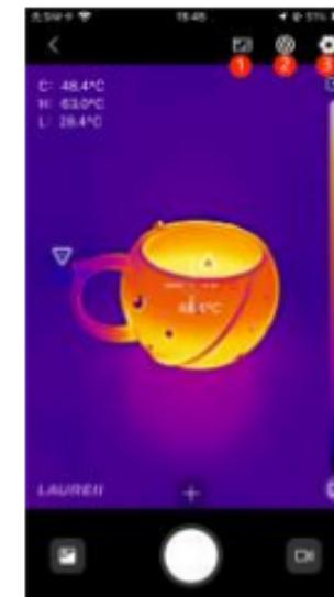
Note: If visible and Thermal do not fully coincide in fusion mode and picture-in-picture mode, you can drag the direction button on the upper right of the image to adjust the horizontal and vertical offset, so that it is aligned with the Thermal horizontal direction.
