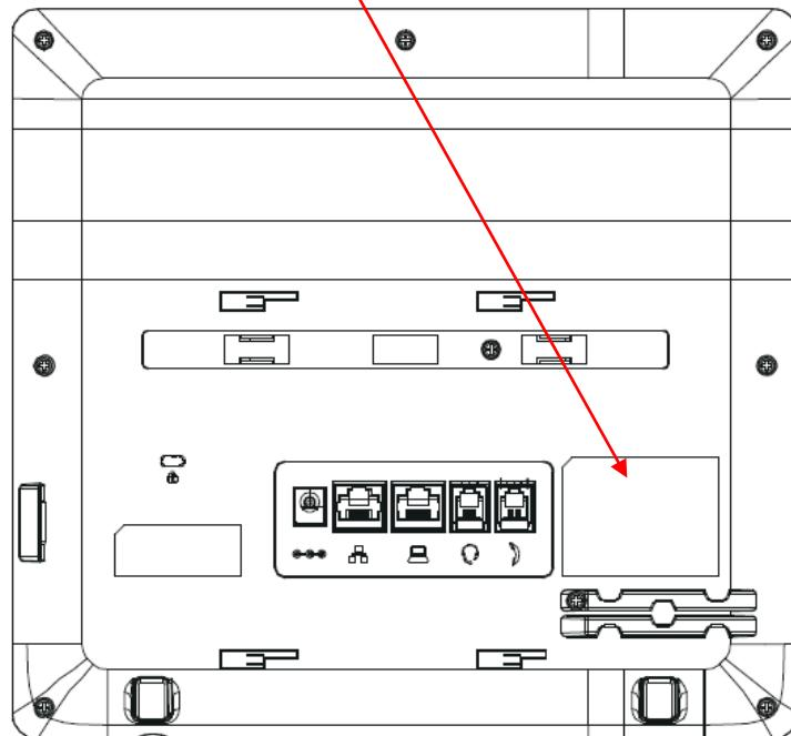
The label shown shall be permanently affixed at a conspicuous location on the device and be readily visible to the user at the time purchase (Labeling requirements per 2.925)
