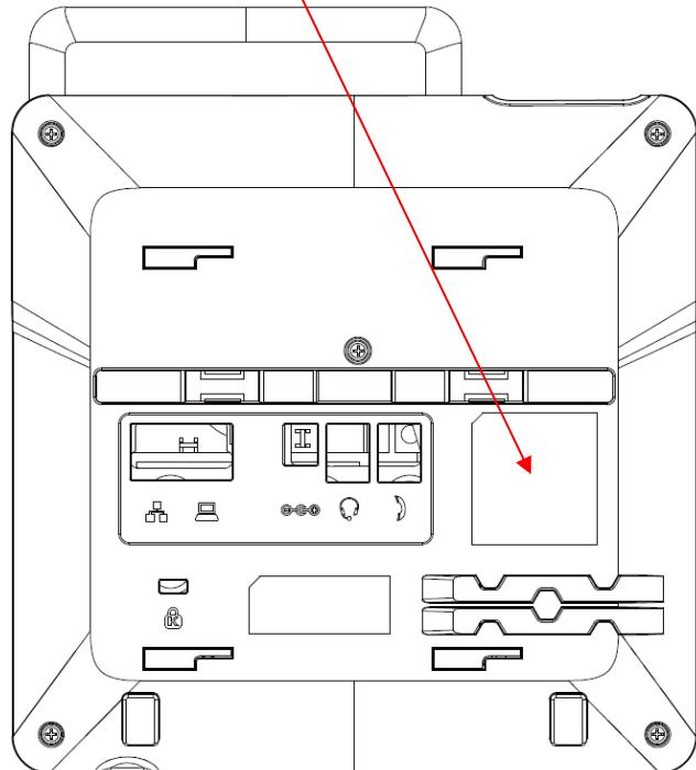
The label shown shall be permanently affixed at a conspicuous location on the device and be readily visible to the user at the time of purchase (Labeling requirements per 2.925)
