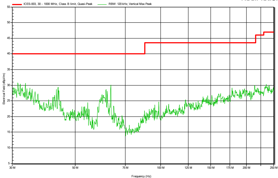
Plot 3c: radiated emissions of the EUT, Antenna vertical, in the range 30 – 250 MHz (pre-scan peak values shown) Low channel IEEE 802.11 b
