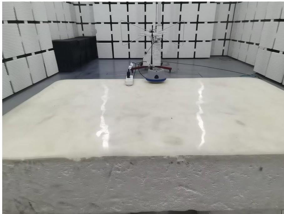
**Set-up for Radiated Emission (RE), Above 1GHz**
