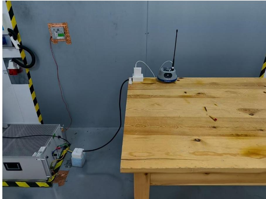
**Set-up for Radiated Emission (RE), Below 1GHz**
