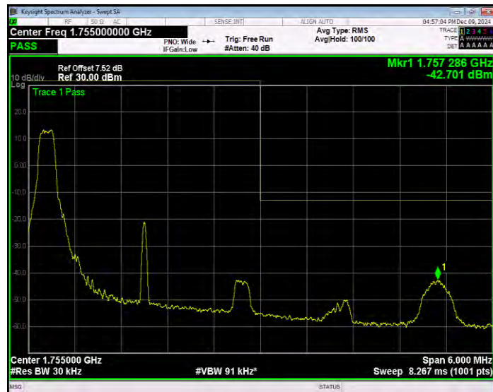
Band4 QPSK BW=3MHz Channel=20385 RB Size=15 Position=#0 Extended
