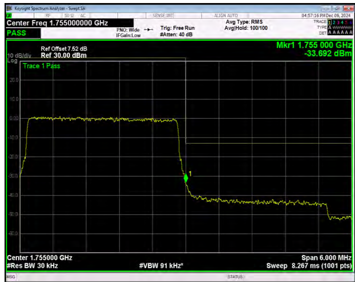
Band4 QPSK BW=5MHz Channel=19975 RB Size=1 Position=#0 Normal
