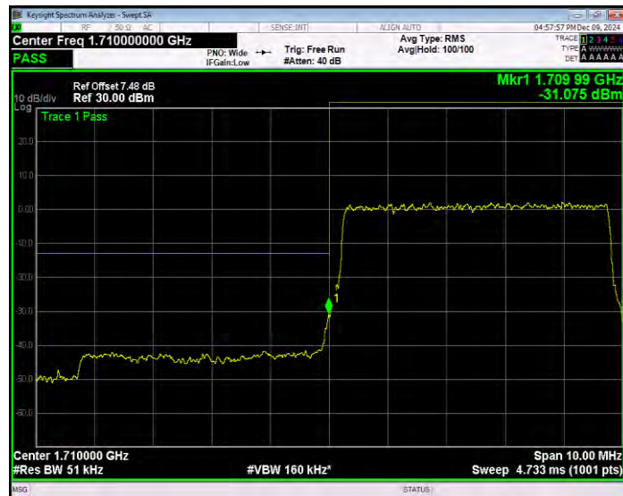
Band4 QPSK BW=5MHz Channel=19975 RB Size=25 Position=#0 Extended
