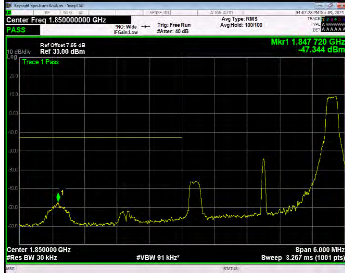
Band2 16QAM BW=3MHz Channel=18615 RB Size=15 Position=#0 Extended
