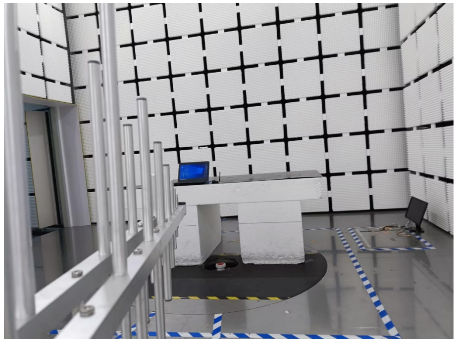
Radiation Emission Test Setup (30MHz to 1GHz)
