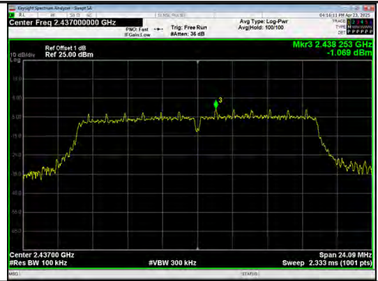
In-Band Reference Level IEEE 802.11g_Channel 6_20MHz_Antenna 0
