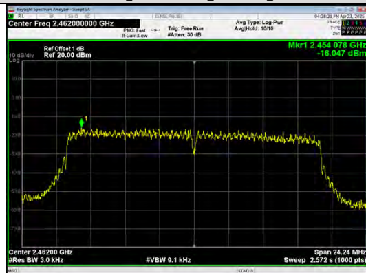
IEEE 802.11n_Channel 1_20MHz_Antenna 0
