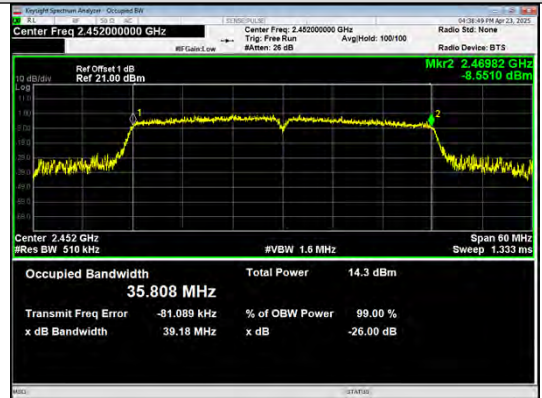
IEEE 802.11n_Channel 9_40MHz_Antenna 0
