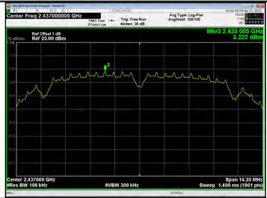
In-Band Reference Level IEEE 802.11b_Channel 6_20MHz_Antenna 0
