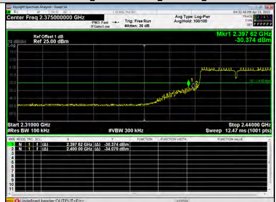
Out Of Band Emission IEEE 802.11n_Channel 3_40MHz_Antenna 0
