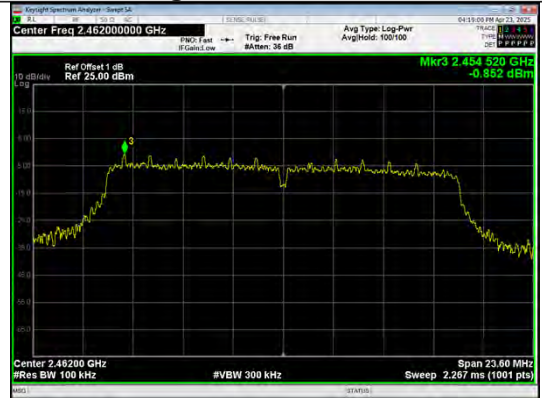
In-Band Reference Level IEEE 802.11g_Channel 11_20MHz_Antenna 0
