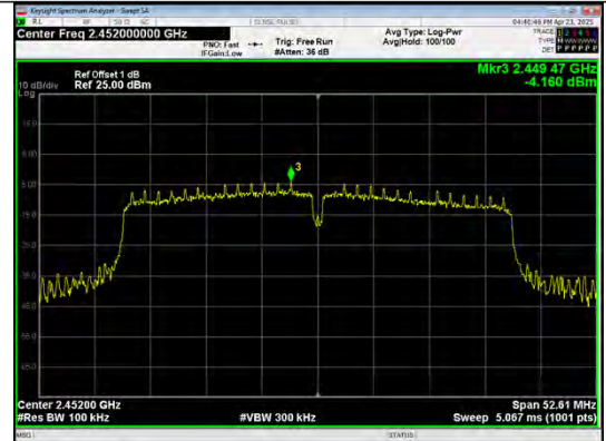
In-Band Reference Level IEEE 802.11n_Channel 9_40MHz_Antenna 0
