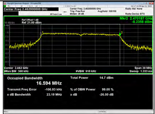
IEEE 802.11g_Channel 11_20MHz_Antenna 0
