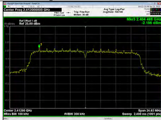
In-Band Reference Level IEEE 802.11n_Channel 1_20MHz_Antenna 0
