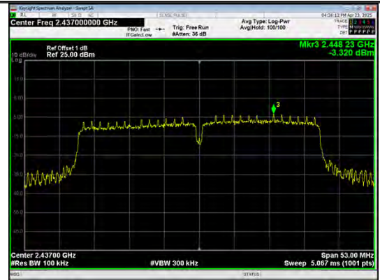
In-Band Reference Level IEEE 802.11n_Channel 6_40MHz_Antenna 0
