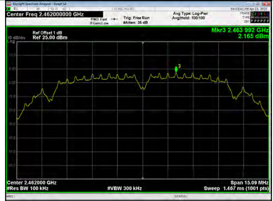
In-Band Reference Level IEEE 802.11b_Channel 11_20MHz_Antenna 0
