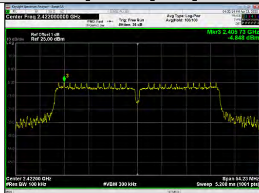
In-Band Reference Level IEEE 802.11n_Channel 3_40MHz_Antenna 0
