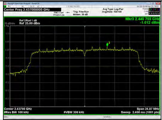
In-Band Reference Level IEEE 802.11n_Channel 6_20MHz_Antenna 0
