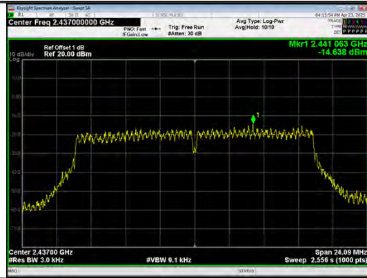
IEEE 802.11g_Channel 6_20MHz_Antenna 0
