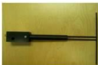
Figure 1 – MVG COMOSAR Validation Dipole
