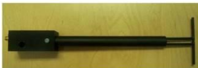
Figure 1 – MVG COMOSAR Validation Dipole
