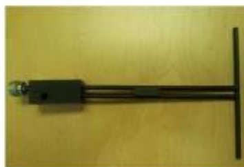
Figure 1 – MVG COMOSAR Validation Dipole
