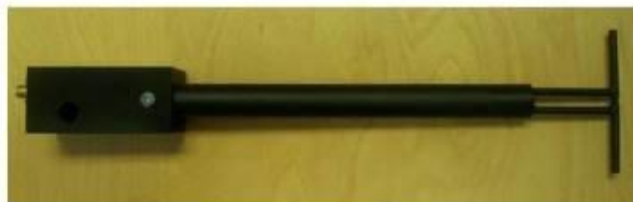
Figure 1 – MVG COMOSAR Validation Dipole
