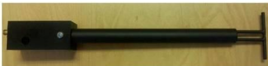
Figure 1 – MVG COMOSAR Validation Dipole
