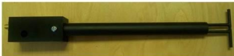
Figure 1 – MVG COMOSAR Validation Dipole
