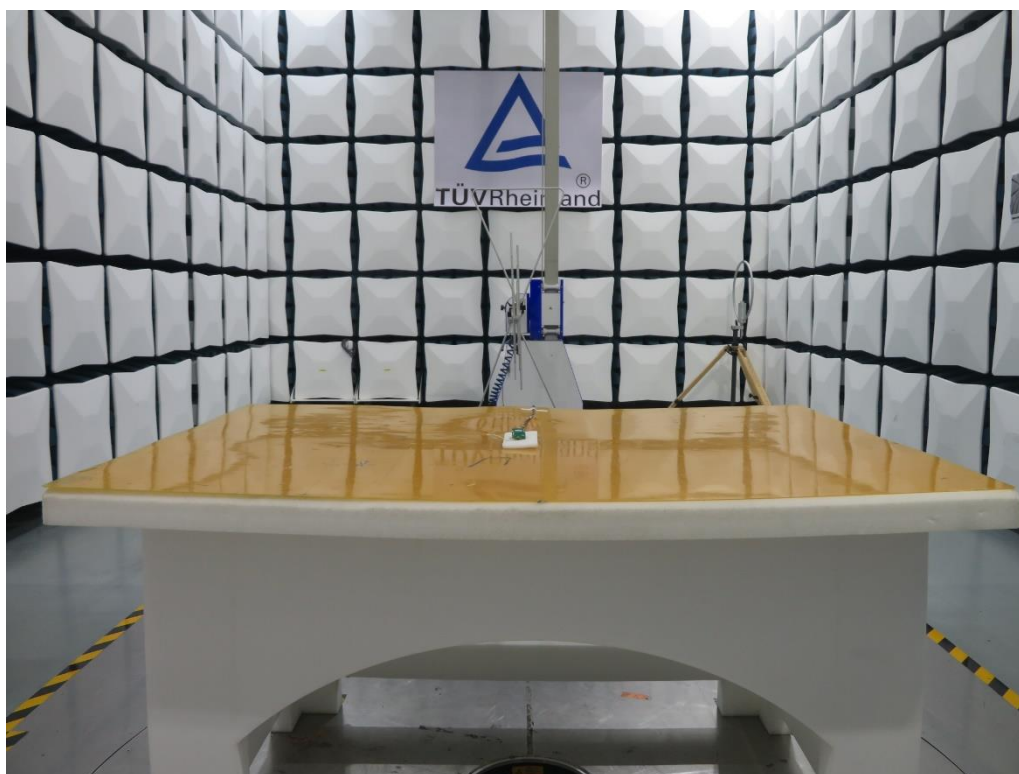
Photograph 1: Set-up photo for Radiated Spurious Emission, below 1 GHz (Ant 1#)
