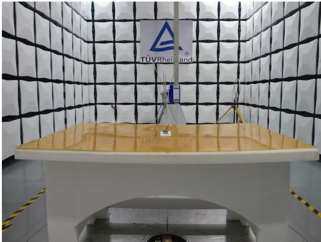
Photograph 5: Set-up photo for Radiated Spurious Emission, below 1 GHz (Ant 3#)
