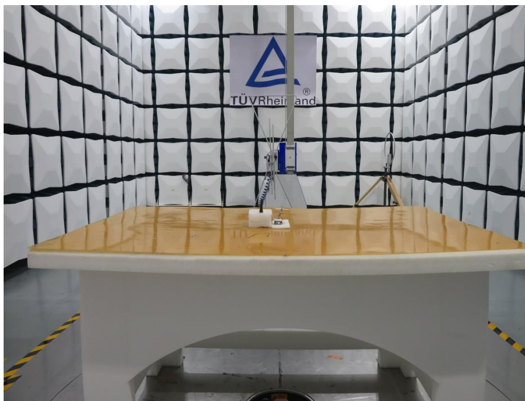
Photograph 3: Set-up photo for Radiated Spurious Emission, below 1 GHz (Ant 2#)
