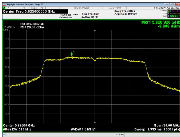
(802.11n20) PSD plot on channel 165
