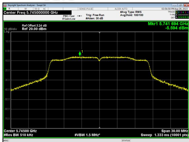
(802.11a) PSD plot on channel 149
