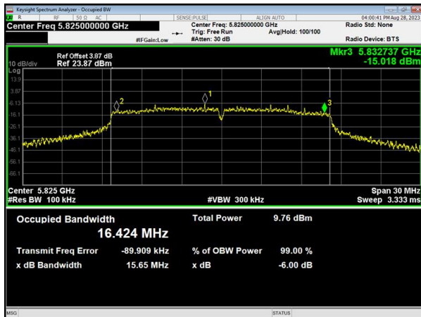
(802.11a) 6dB Bandwidth plot on channel 165
