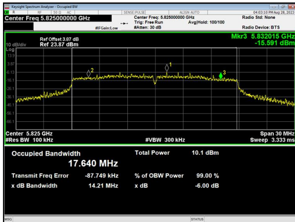
(802.11n20) 6dB Bandwidth plot on channel 165
