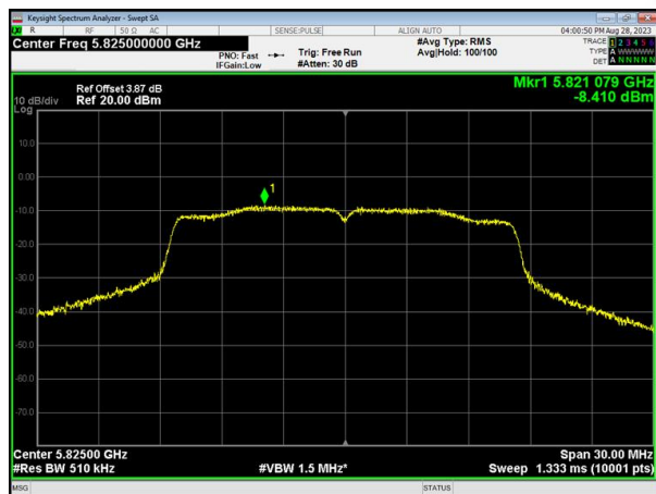
(802.11a) PSD plot on channel 165
