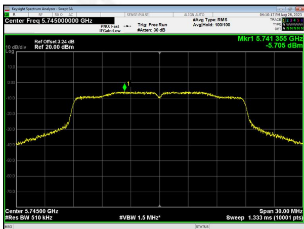
(802.11ac20) PSD plot on channel 165
