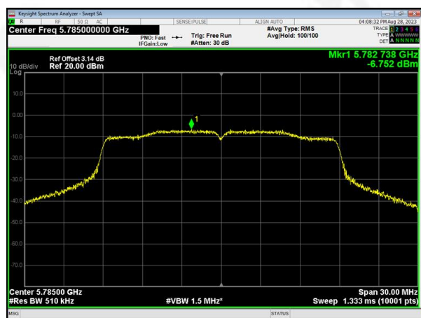
(802.11ac20) PSD plot on channel 157
