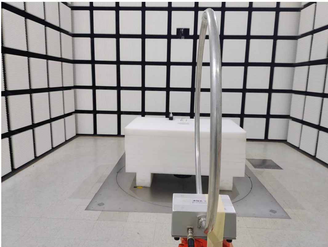
Radiated Emission 9k-30MHz Perpendicular View
