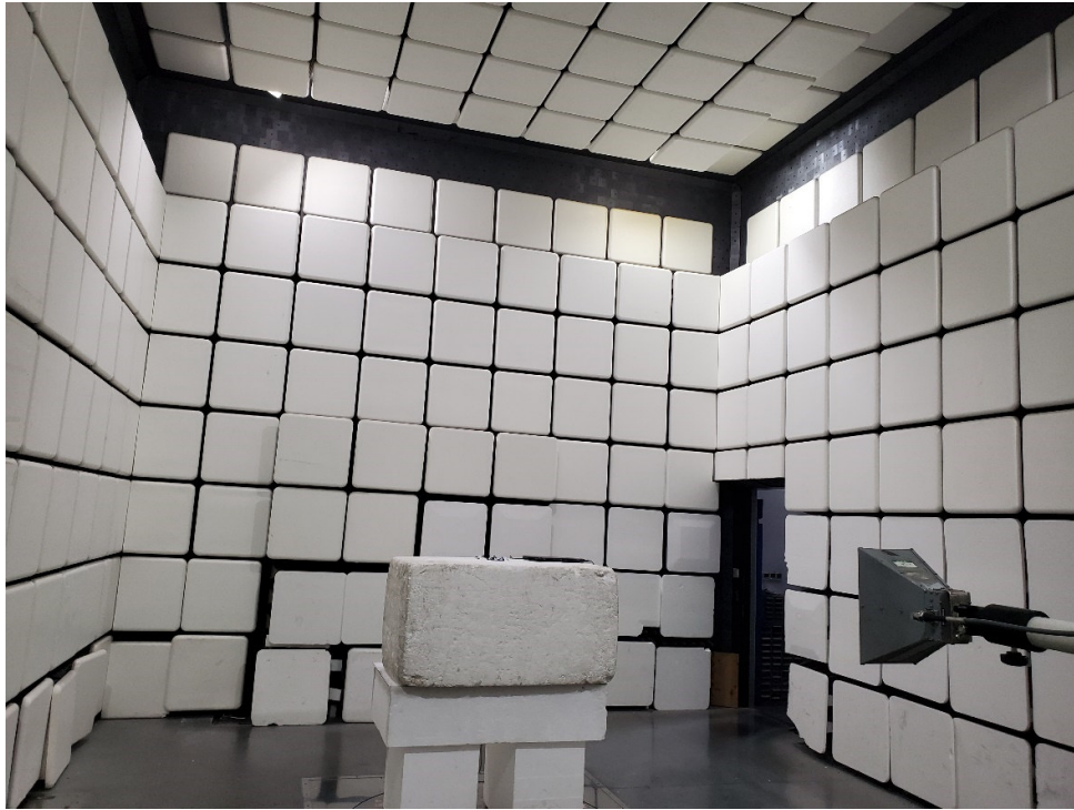
Picture 1 Radiated Emission Test Setup
