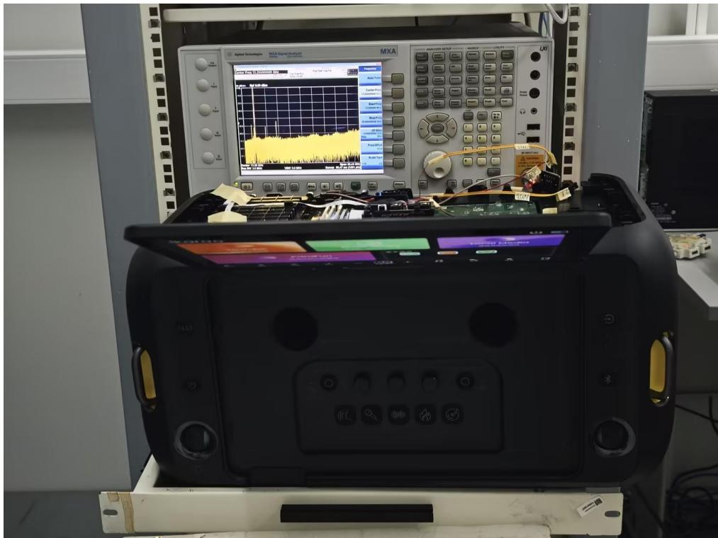
**2.4G ANT 5 RF CONDUCTED TEST SETUP**
