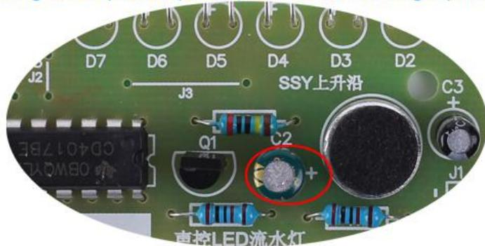
Step 12: Install the extra pins from LED at J1-J3.
