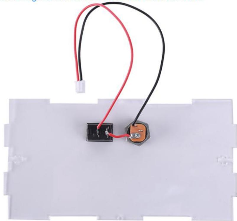
Step 27: Connect 1pcs power wire to red socket and 2pcs speaker wires to white sockets.
