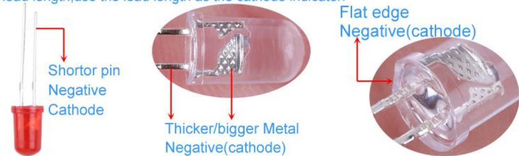
Step 6: Install 10pcs 5mm RGB LED at D1-D10. Pay attention to distinguish between positive and negative at Step5 and bend the LED pins.
