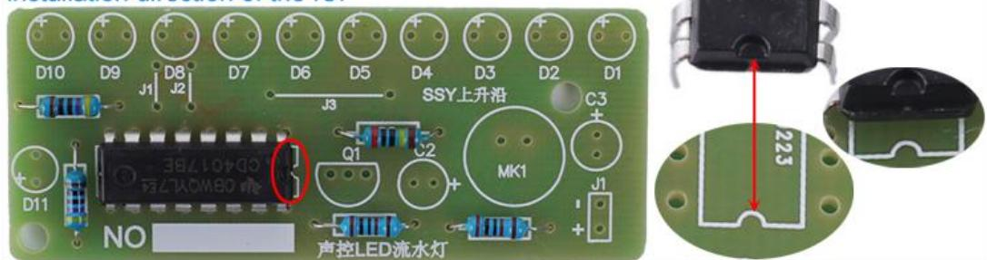
Step 5: Identify the positive(anode) and negative(cathode) lead of LED. The leads of the LED must be installed correctly, otherwise the LED cannot be turned on. Here are four methods as following:
