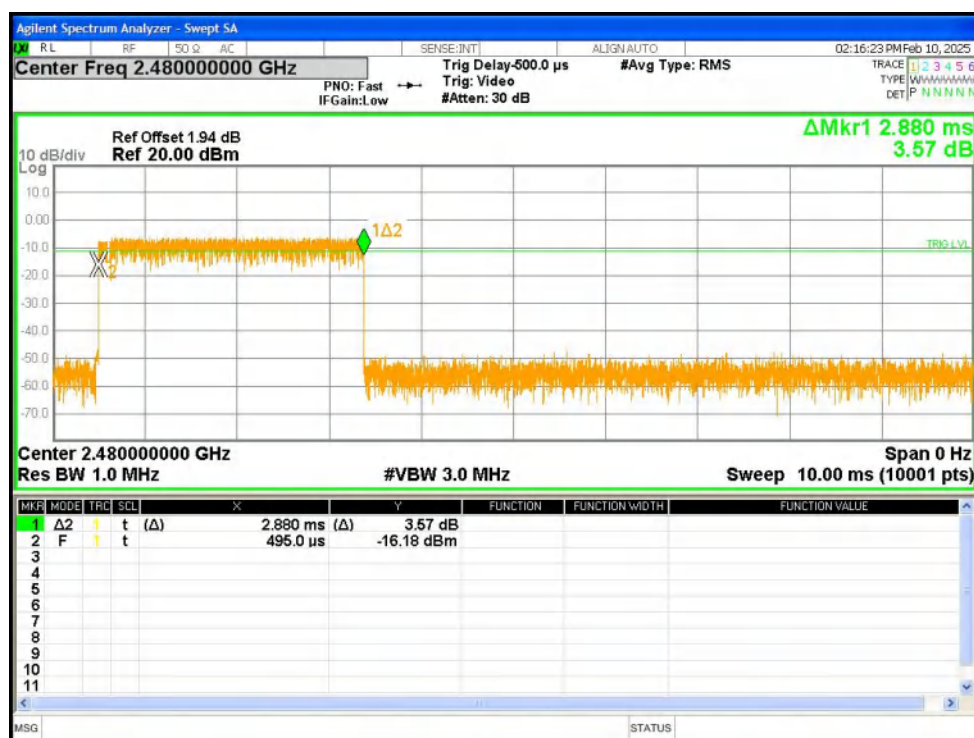
Dwell NVNT 3-DH5 2480MHz Ant1 One Burst
