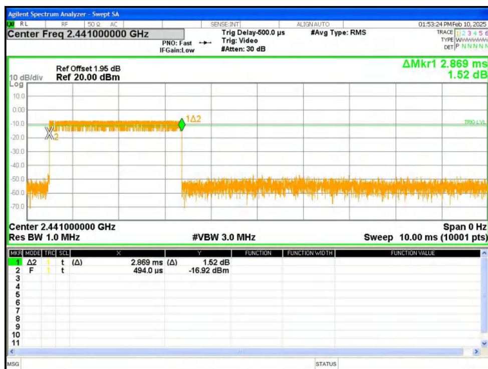
Dwell NVNT 1-DH5 2441MHz Ant1 One Burst
