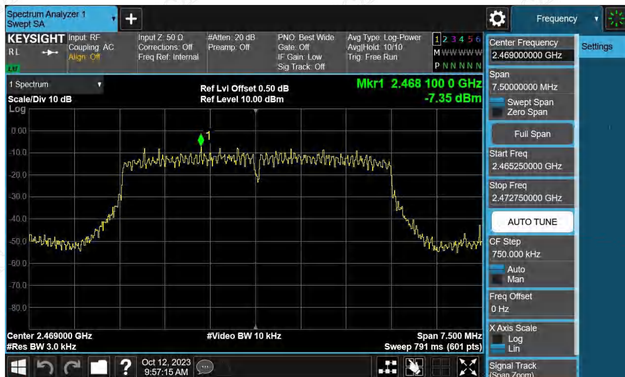
Figure 9: Power Spectral Density, Bandwidth 5MHz, 2469MHz
