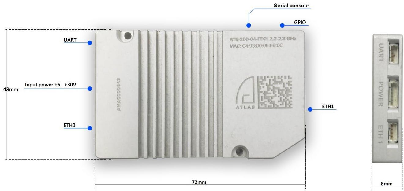
The carrier board above has 2x100 Mbit/sec transformer less ethernet interfaces, one high speed UART port (up to 1 Mbit/s) to connect to AtlasPRO UAV autopilot, one I2 C temperature sensor connected via USB IO extender (based on STM32 MCU), one GPIO button for radio modules pairing, one serial console for debugging purposes and single input power connector. IO extender is a composite USB device with two interfaces:
