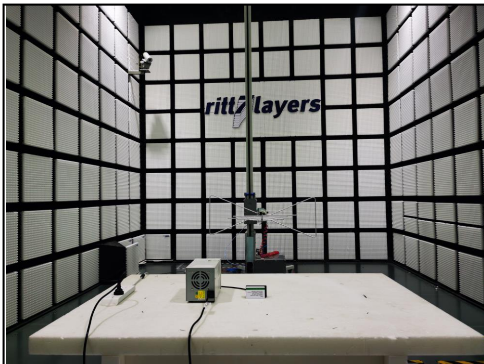
Fig. 2 Radiated emission setup photo(30MHz-1GHz)
