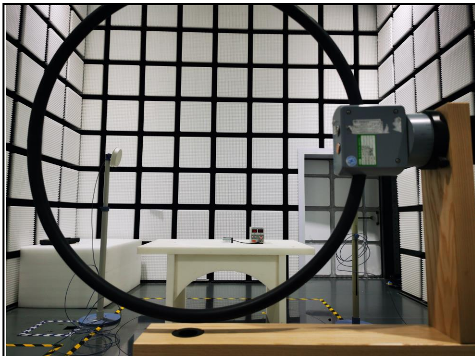
Fig. 1 Radiated emission setup photo(Below 30MHz)
