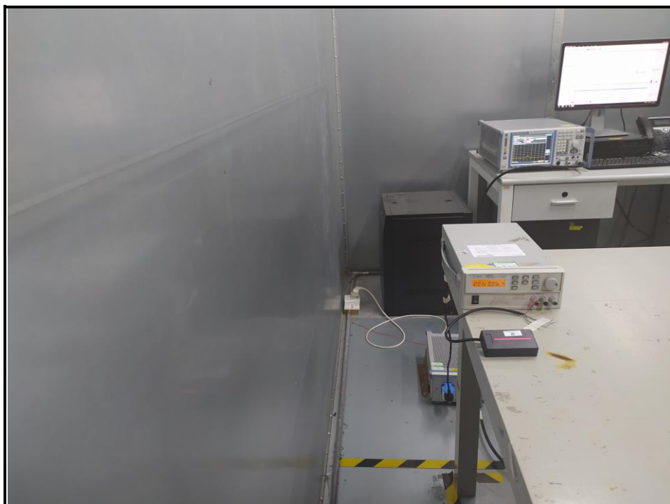
Fig. 4 Power line conducted emission setup photo
