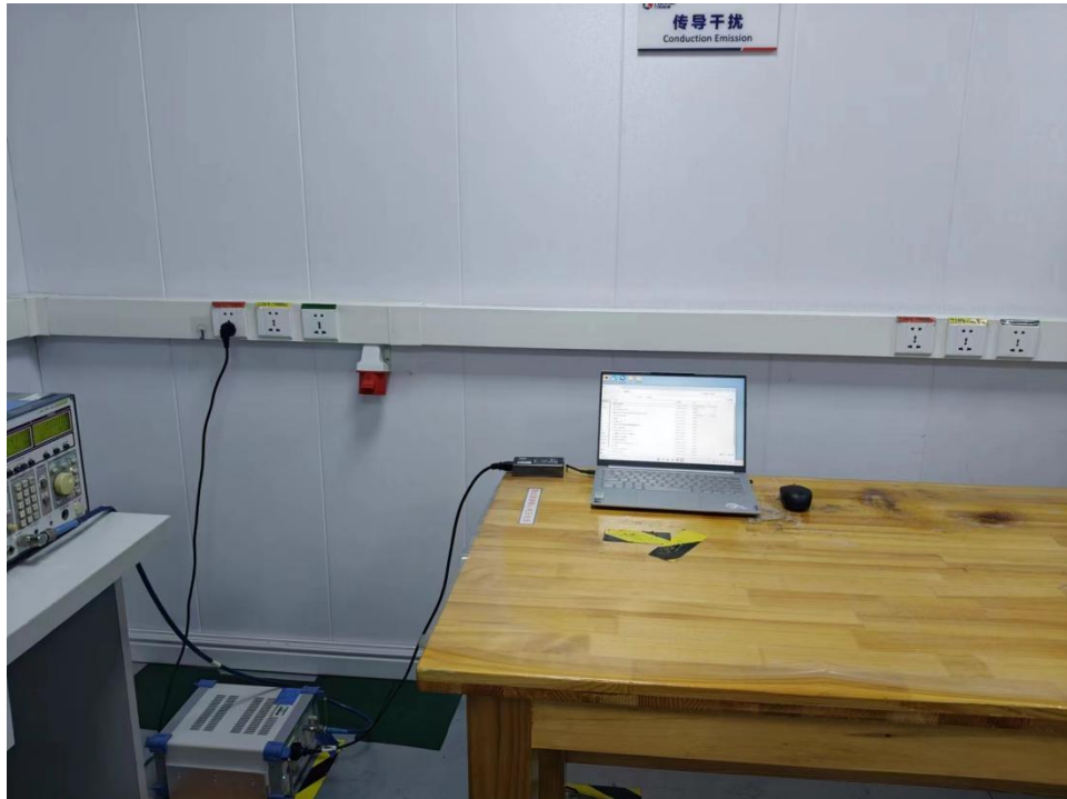
Photograph 3: Set-up for Conducted Emission on AC Mains
