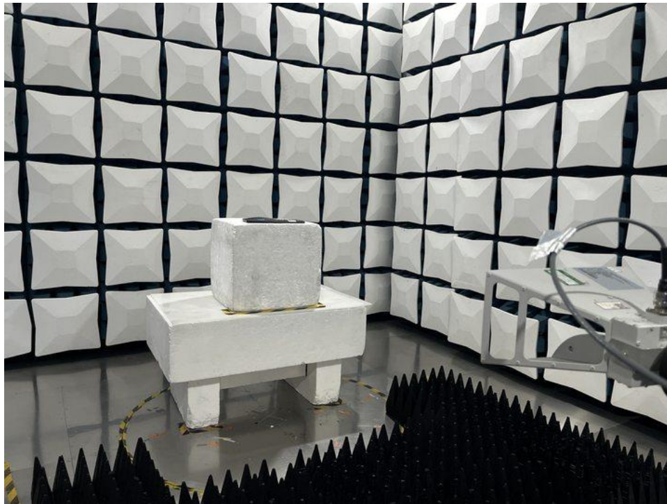
Photograph 2: Set-up for Radiated Spurious Emission, Above 1GHz
