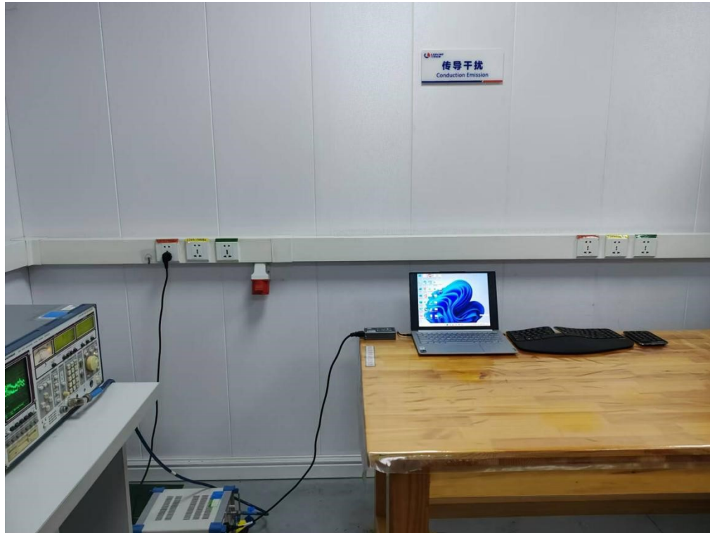
Photograph 3: Set-up for Conducted Emission on AC Mains
