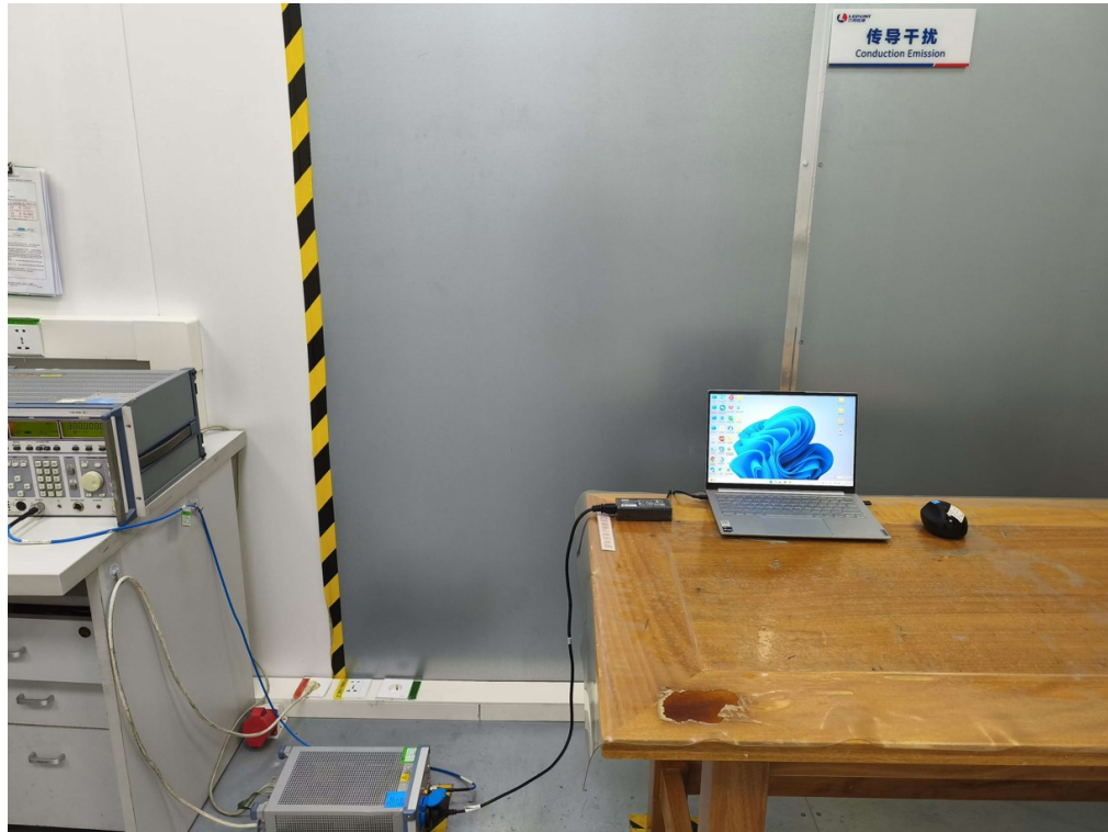
Photograph 3: Set-up for Conducted Emission on AC Mains
