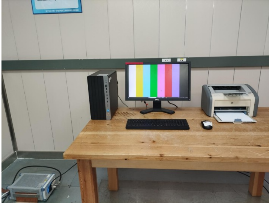
Photograph 3: Set-up for AC Main Conducted Emission
