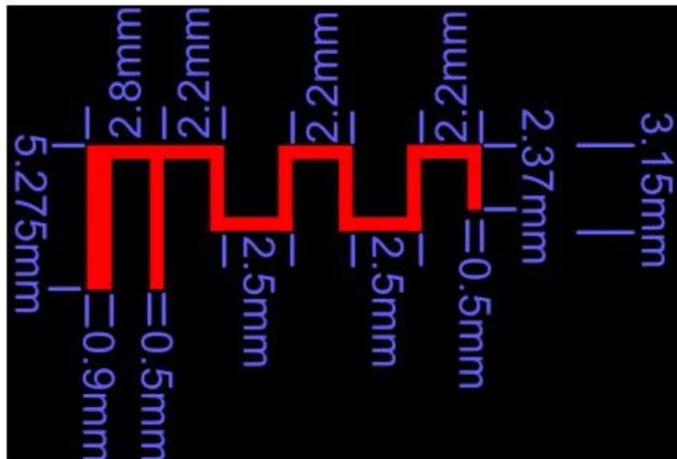
PCB Antenna Size
