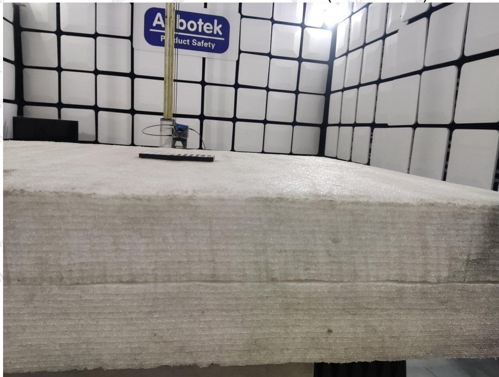
Photo of Radiation Emission Test (above 1GHz)
