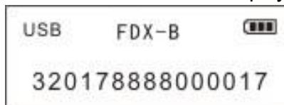
Press and hold the button for 3 seconds to upload the data stored in the device. A maximum of 1024 pieces of data can be uploaded. After the data is uploaded successfully, the interface is as follows.
