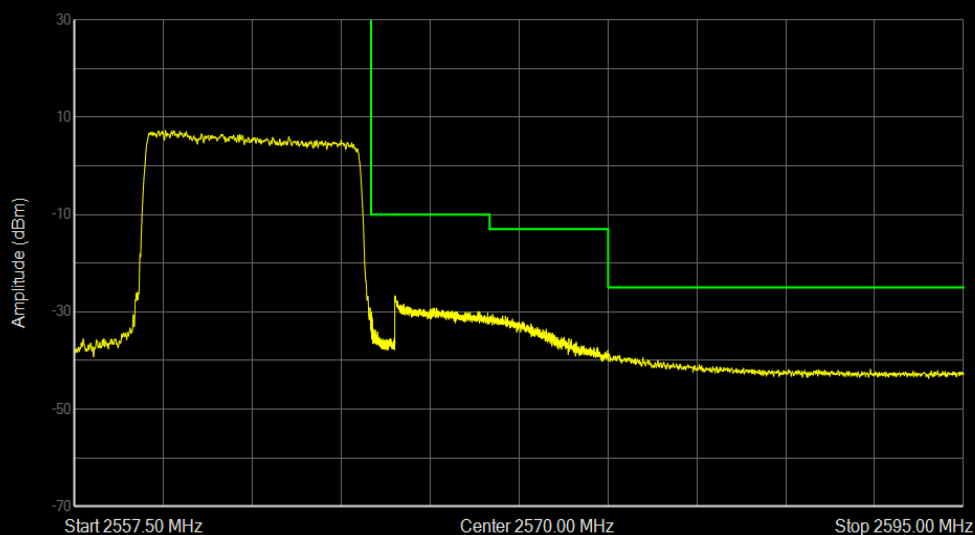
Band7 QPSK BW=10MHz Channel=21400 RB Size=50 Position=#0 NVNT
