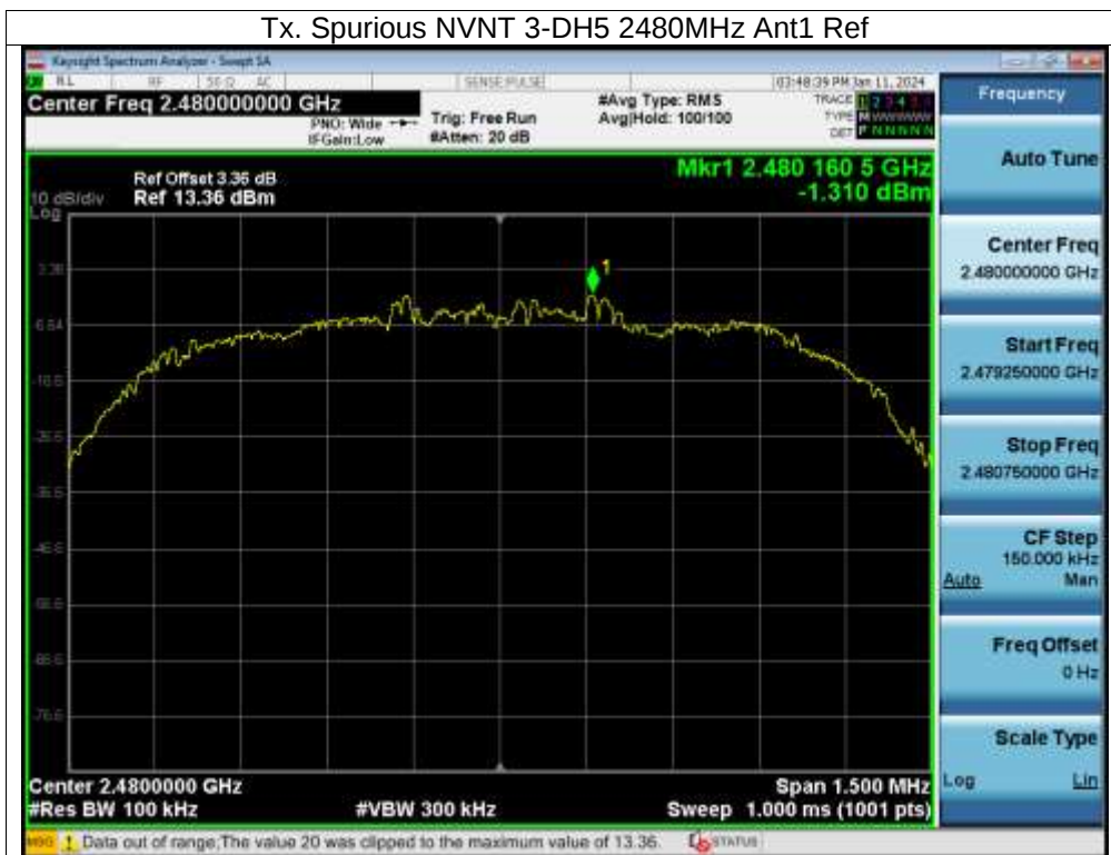
Tx. Spurious NVNT 3-DH5 2480MHz Ant1 Emission
