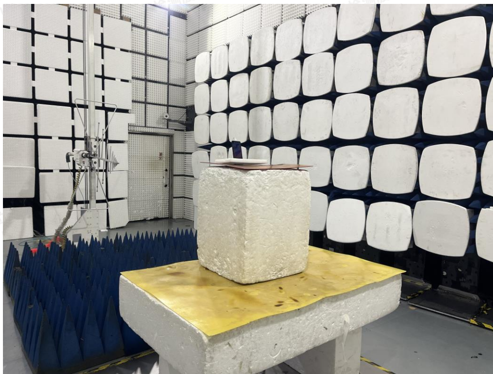
Radiated Emissions Measurement (Below 1GHz)
