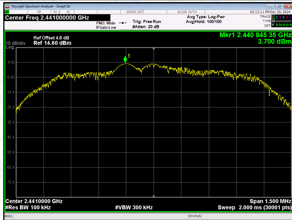
Tx. Spurious NVNT 2-DH1 2441MHz Ant1 Emission
