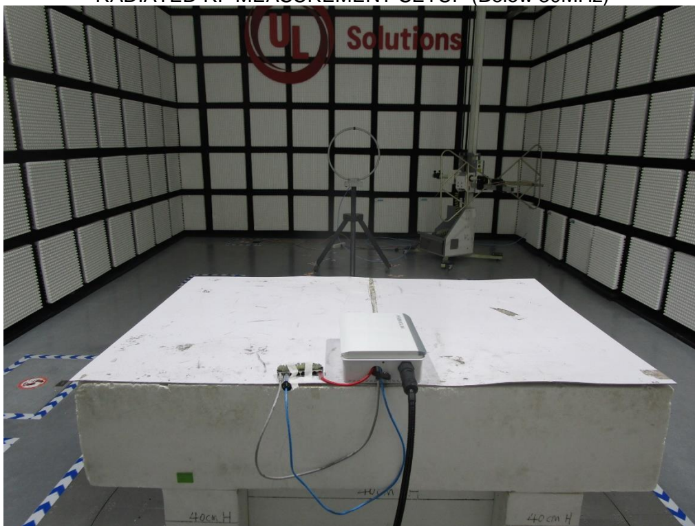
RADIATED RF MEASUREMENT SETUP (Below 30MHz)
