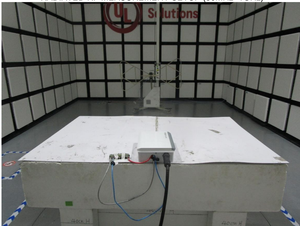
RADIATED RF MEASUREMENT SETUP (Below 30MHz)
