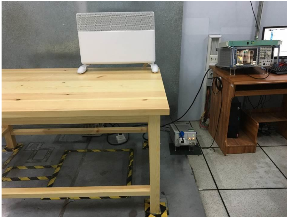
Test Setup For Conducted Emission
