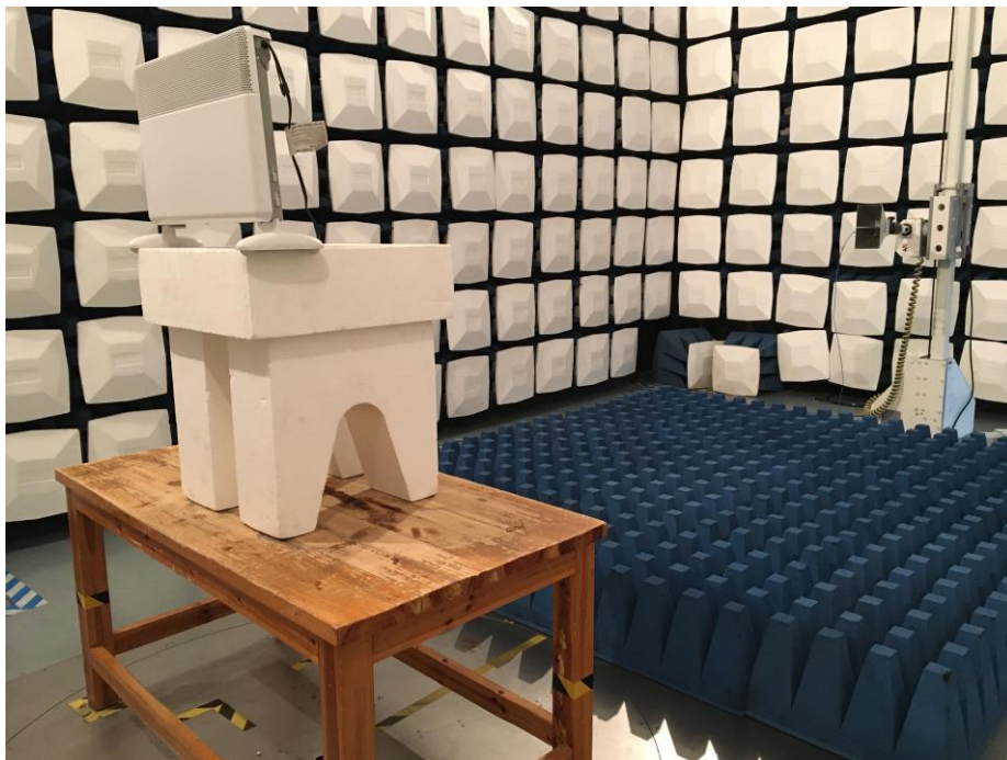
Test Setup For Radiated Emission (Above 1GHz)
