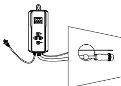
C: Please pass the power cord through the drilled hole, and then hang the controller in a suitable place. Then hang the controller in a suitable place (the controller is waterproof to IP55, try to avoid long-term use in the rain).
