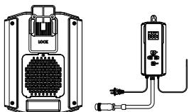
D: Installation of the controller power cord: connect the power cord with the host power hole, and then tighten the nut on the power cord clockwise.
