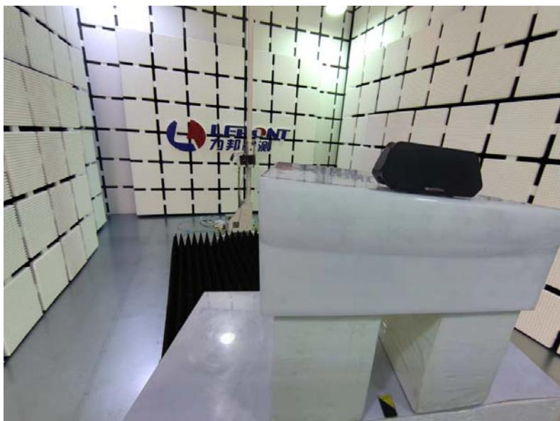
Conducted disturbance at mains terminals Test
