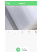
2-3. After connecting the camera, return to the APP and refresh the page to show the device that the proximity mode is successfully connected. (Range is only within 10 meters)
