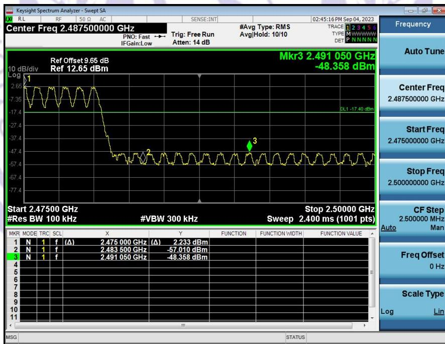
$\pi/4$ -DQPSK No-hopping Band edge-left side
