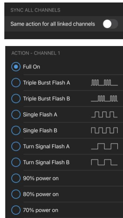
**Sync All Channels-** Each channel can perform different actions on the same sensor wire. Select this option to sync all channels.
